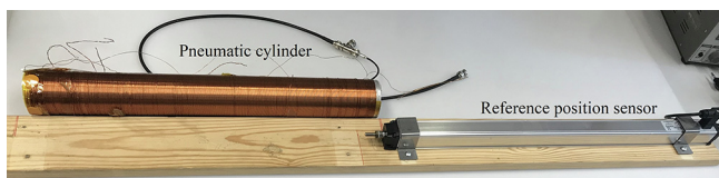
Fig. 5. Pneumatic cylinder and reference position sensor.
