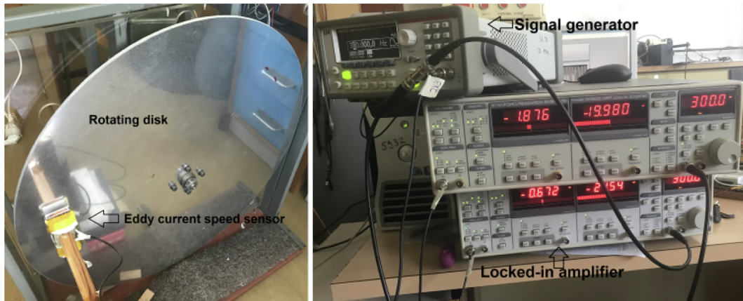
Fig. 3. Experimental set up – rotating disk (aluminum and solid iron) as moving part and eddy current based speed sensor (left) and signal generator and lock-in amplifier (right).
