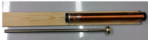
FIG. 2. Piston and piston rod of the model cylinder.
