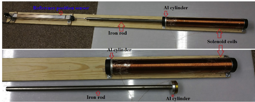
Fig. 12. Measurement set-up for a pneumatic position sensor.
