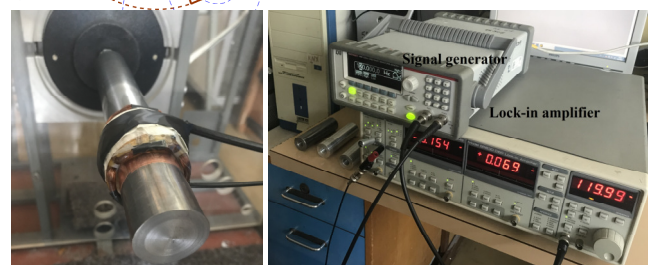
Fig. 6. a) Schematic block diagram for speed measurement (top) and b) an eddy current speed sensor mounted on the rotating solid iron rod and a signal generator and a lock-in amplifier (bottom)
